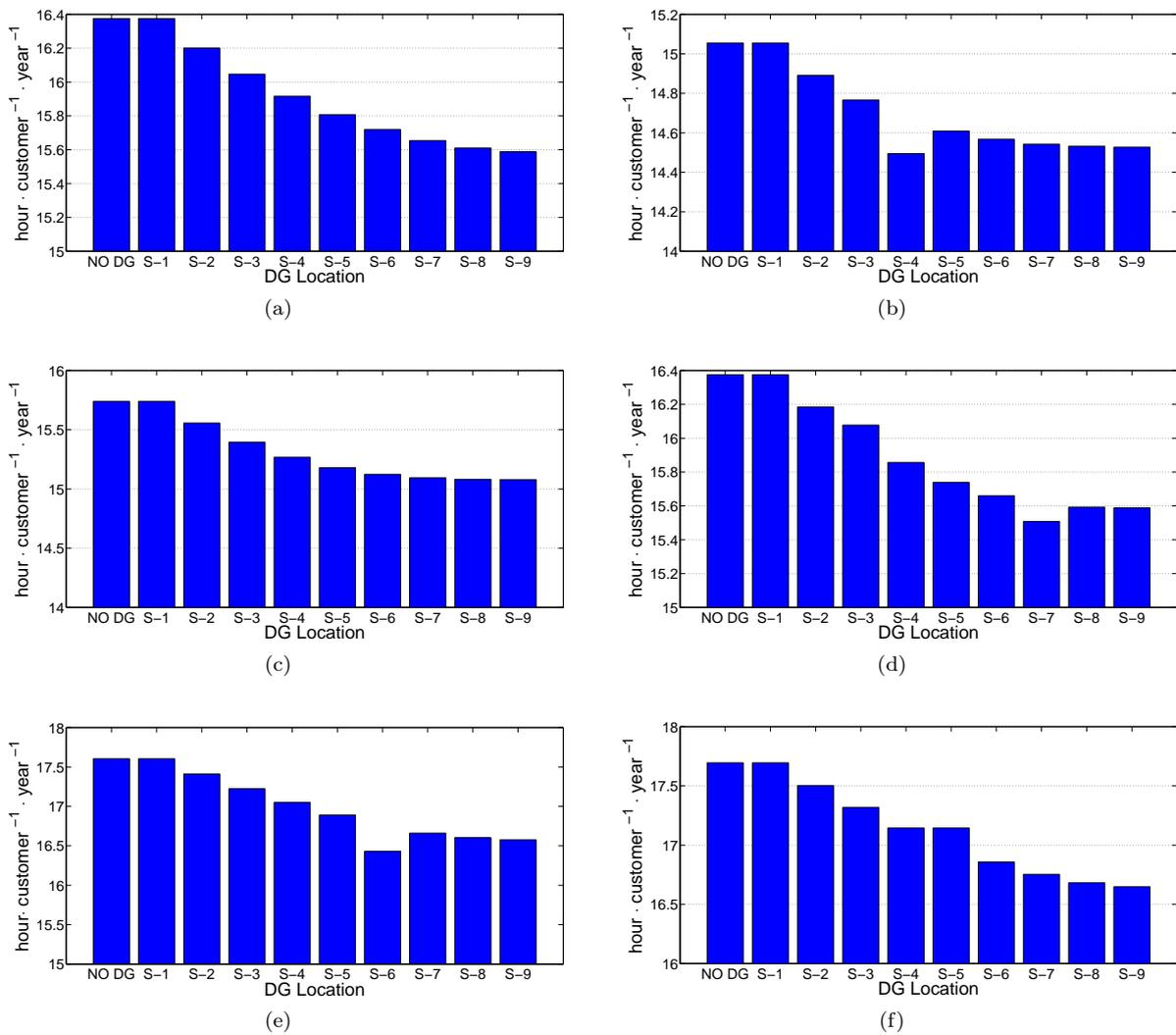
**Fig. 6:** (a) SAIDI for customer scattering case-1, (b) SAIDI for customer scattering case-2, (c) SAIDI for customer scattering case-3 (d) SAIDI for customer scattering case-4, (e) SAIDI for customer scattering case-5, (f) SAIDI for customer scattering case-6.
